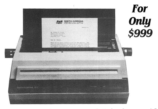
Ideally suited for small businesses or the home user, the TP-1 is a microprocessor controlled, correspondence quality printer that prints fully formed characters at an average print speed of 12 characters per second. This simple to operate, compact printer is compatible with most microcomputers and comes with the standard Centronics parallel interface (an optional serial data interface is available) and features:
